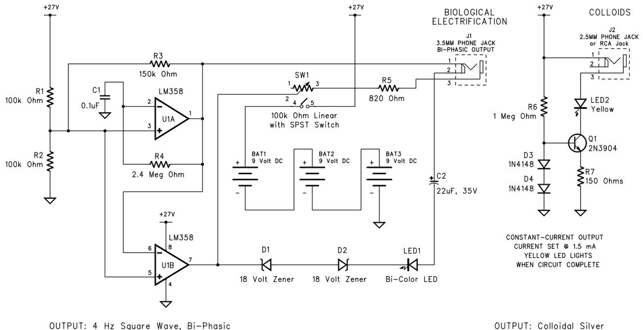
Note: This schematic uses the Constant Current Method to make the ionic colloidal silver.
