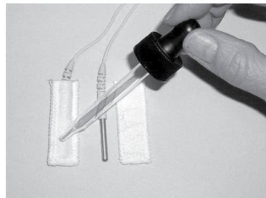
**Step 2:** Place the cotton sleeves over the electrodes. A dropper bottle is a handy way to wet the cotton and to keep the covers damp during use.
